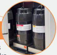
NoeCha ROLL2-S uses NoeCha Sublimation inks which are stored in **20-litre containers** directly connected to the ink system. A scale under each container allows an easy control of the ink levels.
